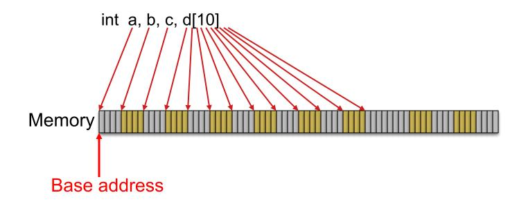
Each word is referred to with the address of a single byte
