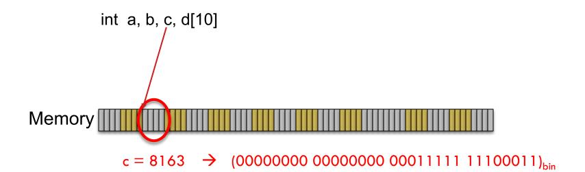
Each word is referred to with the address of a single byte
